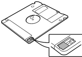
When the tab window is open, formatting and recording are not possible.
