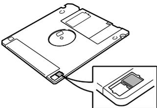
When the tab window is closed, formatting and recording are possible.
