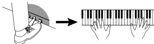
A pedal count-in can be any number of beats. Press the sustain pedal as many times as necessary; each press will be recorded as a count-in beat.
