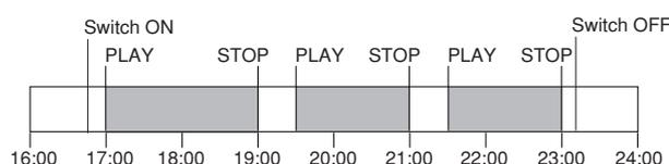
The Disklavier above is set to play songs continuously from 5:00 p.m. to 11:00 p.m., with interruptions for live performances at 7:00 p.m. and 9:00 p.m. for 30 minutes each.
