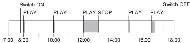
The Disklavier above is turned on at 7:55 a.m., and Timer Play starts at 8:00 a.m. with the opening of the store. Songs are set to be played at 8:00 a.m. for the opening of the store, at 10:00 a.m. and 3:00 p.m. to signify the time, during lunch, and at 5:00 p.m. for the closing of the store.
