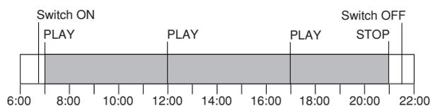
The Disklavier above is set to play at 7:00 a.m., 12:00 p.m. and 5:00 p.m., and set to stop at 9:00 p.m. At each of the specified time, it plays a group of songs until all the disks in the group are played back. The Disklavier will stop playing at 9:00 p.m. even if Grp3 is still playing.
