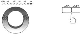
Tuning adjustments can be made from -050 to +050 in 1 cent steps (100 cents equals 1 semitone).
