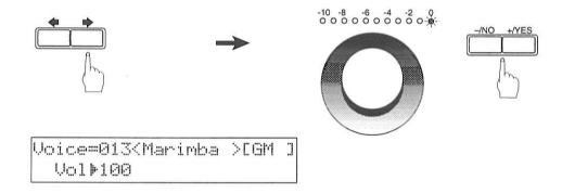
Note: In Voice mode, the volume of the parts you play on the keyboard is set by the Vol parameter and is not affected by TG Master Balance or the volume Dial on the front panel.
