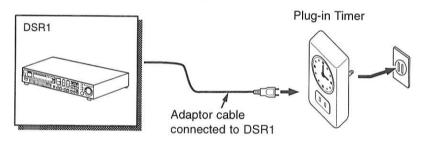
Note: Be sure to switch off the DSR1 first, and wait at least 5 seconds before disconnecting it from the AC outlet. Otherwise, volume and balance settings may be altered to inappropriate settings when the DSR1 begins Auto Start.
