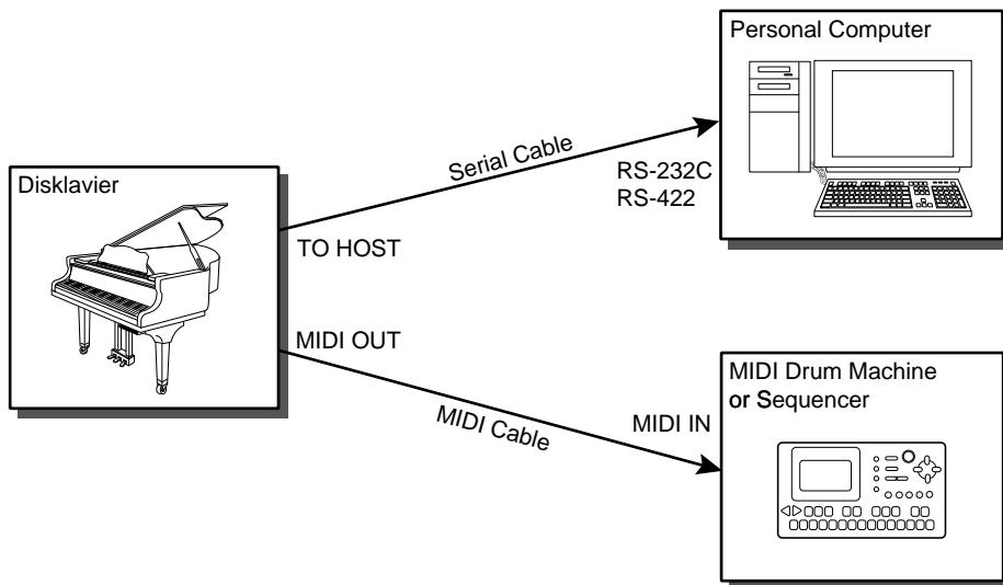
**Note:** To use the Disklavier properly with the computer setups described in this chapter, it is recommended that you connect your computer to the TO HOST connector and set the HOST SELECT switch to PC1, PC2, or MAC depending on your computer type. See “Setting the HOST SELECT Switch” on page 72.
