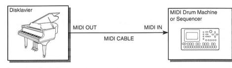
Set the MIDI drum machine or sequencer to synchronize with the incoming MIDI clock, sometimes called "MIDI SYNC". Refer to its operating manual for details.
