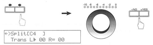
The MIDI output can be transposed from -60 to +60 in one semitone steps. Separate transposition values can be set for the left- and right-hand parts.
