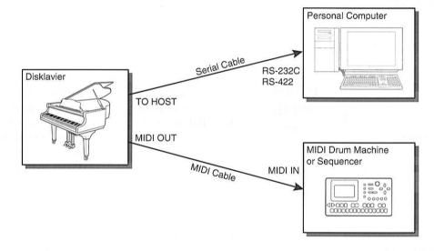
Note: For the computer setups described in this chapter, it is recommended that you connect your computer to the TO HOST connector and set the HOST SELECT switch to PC1, PC2, or MAC depending on your computer type, so that the Disklavier functions properly. See "Setting the HOST SELECT Switch" on page 83.
