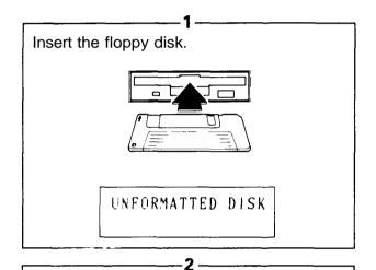
After inserting a disk, press the Rec. button while keeping the Stop button depressed. You can release these buttons when the display reads "FORMAT OK?".
