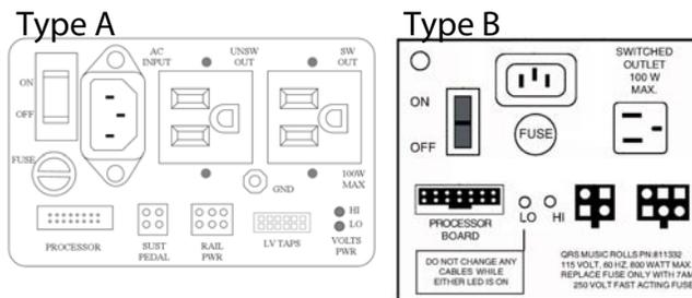
The Power Supply [Type A or B above] and the Processor are located in these areas.
