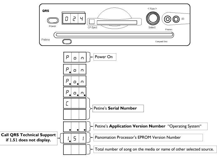
If Petine's "power-on" display sequence is different than what is shown here, see the "Restoring Petine's Operating System" section of this manual.
